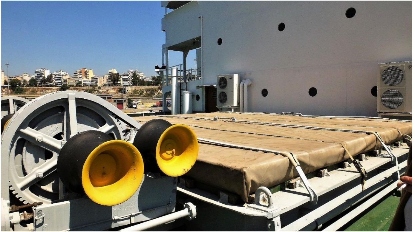
2015. The tarpaulins, the wedges and the new tarpaulin securing bars, on the HELLAS LIBERTY in Piraeus.
